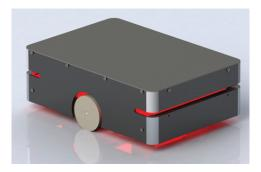
RM100, is a collaborative mobile platform that brings human-robot interaction for material handling in manufacturing and warehousing industries. Capable of carrying a payload on 100Kg, RM100 can autonomously navigate in a human populated environment using constant human detection and obstacle avoidance protocols.
